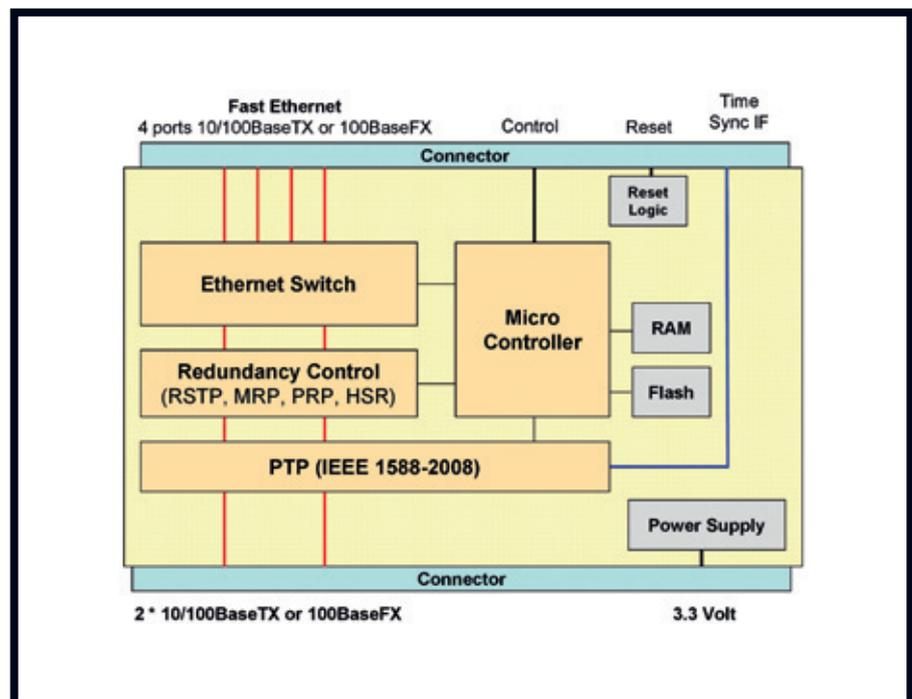
Fig. 3 Block diagram of embedded Ethernet system
